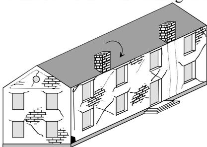
Figure 7. Typical damage of masonry building.
