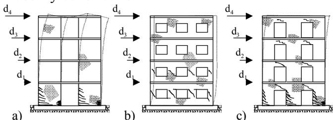
Figure 8. Typical mechanisms of behavior of masonry shear walls (after Tomažević 1999)
