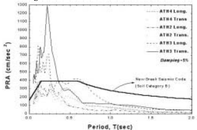
Figure 1. Acceleration response spectra (horizontal components) of the September 7, 1999 earthquake in Athens and elastic design spectra of the Greek Seismic Code.
