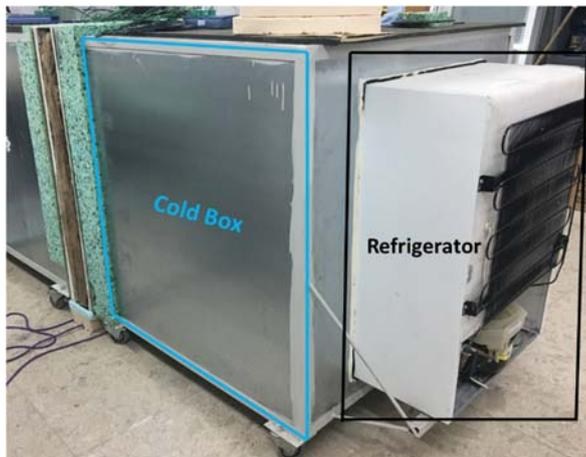
b) Refrigerator attached to the cold box
