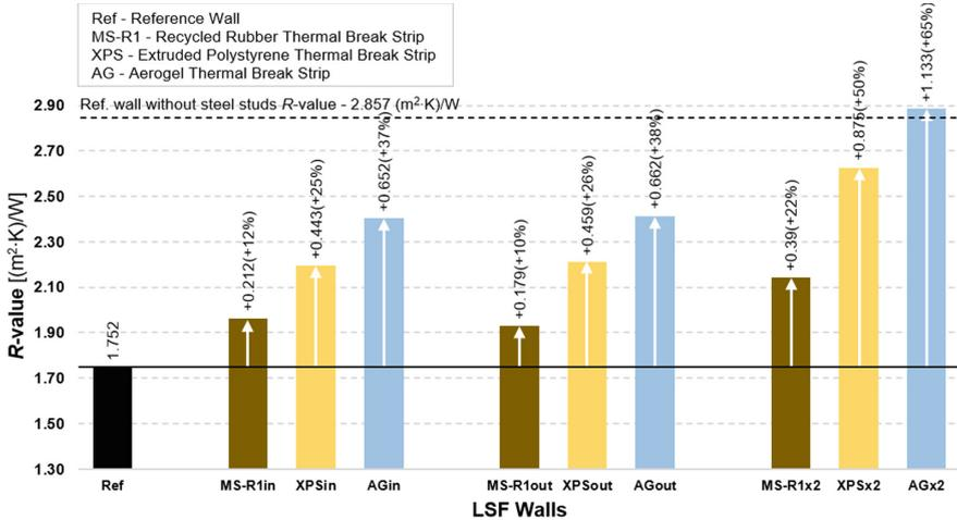
Fig. 5. Measured thermal resistances (conductive  $R$ -values).
