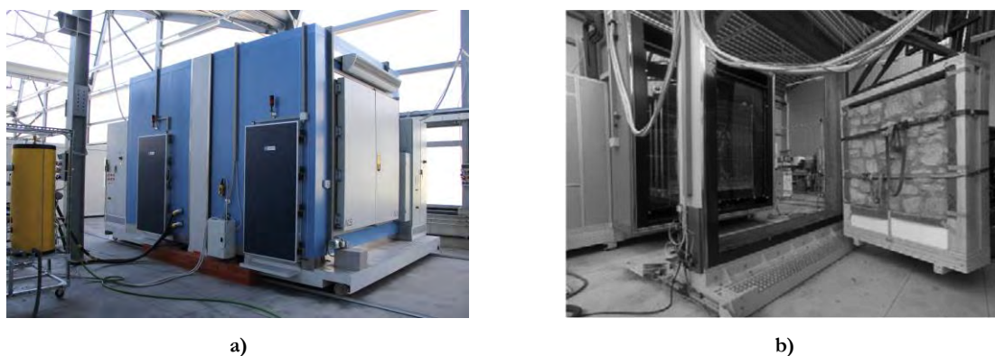
Figure 2.86 – Guarded hot box test: a) apparatus [229]; b) specimen [230].
