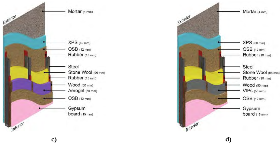
Figure 5.19 – Models with the combined improvement strategies: a) Model H; b) Model I; c) Model J; and d) Model K.
