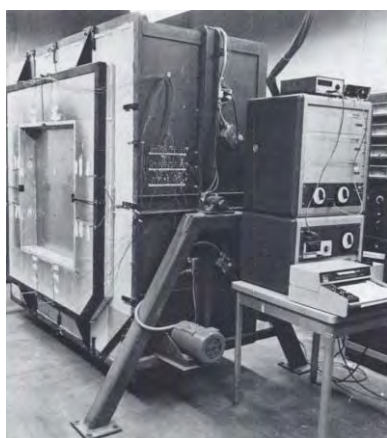
Figure 2.38 – High-temperature guarded hot box: a) vertical cross-section; b) facility photography [161].
