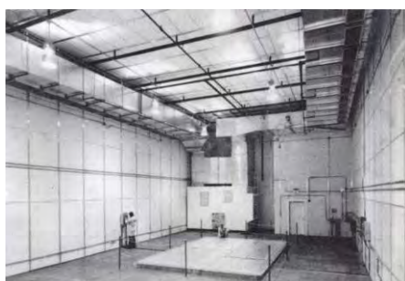
Figure 2.45 – Calibrated hot box apparatus interior of Thermal Research Facility [166].
