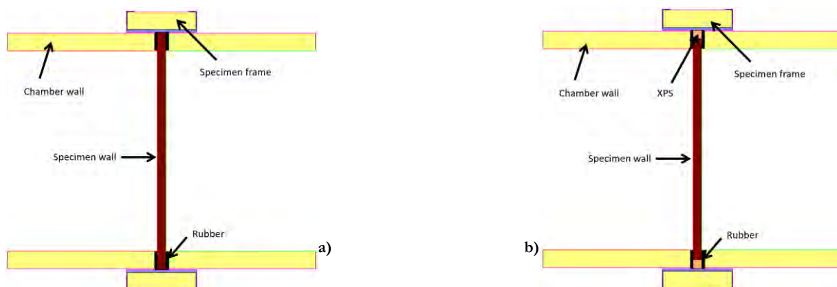
Figure 4.24 – Numerical models of the specimen placed directly: a) on the specimen frame; b) surrounded of insulation with 100 mm.
