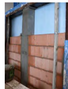
Figure 2.74 – GHB: wall specimen being assembled in the frame [210].
