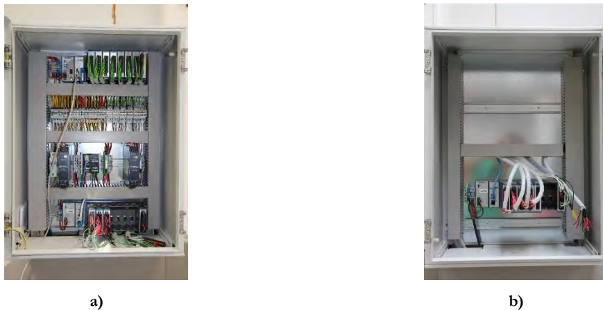
Figure 4.17 – Control and data logging panels: a) main with CompactRIO Controller model cRIO-9074 on the top and the expansion unit NI 9144 8-slot in the bottom; b) secondary with the other expansion unit NI 9144 8-slot.
