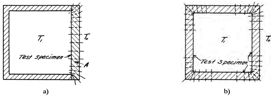
Figure 2.21 – Hot Box method: a) testing over one open side; b) testing a complete cubical of the material [28].
