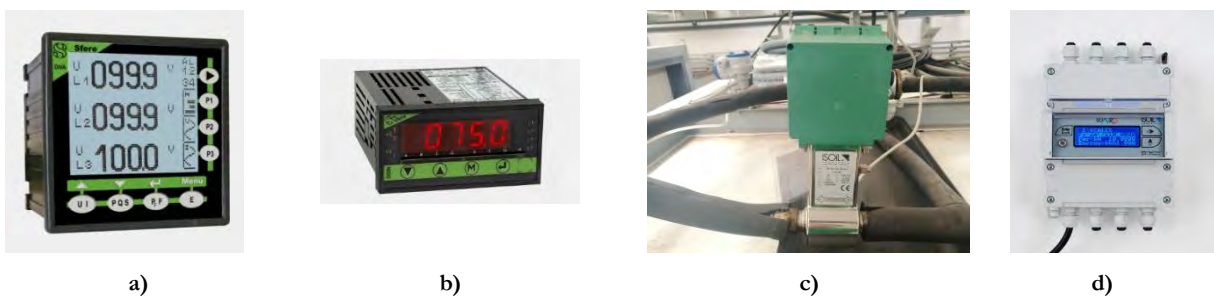
Figure 4.15 – Electric analysers: a) triphasic Sfere model Diva 11 [285]; b) Sfere model Diva 5 [286]; c) Electromagnetic flowmeter; and d) Heat meter integrator.
