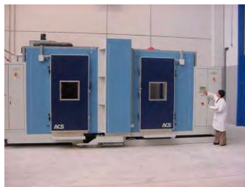
Figure 2.70 – Guarded/calibrated hot box [202].
