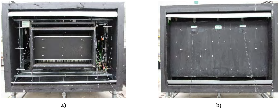
Figure 4.10 – Sensors a) GHB metering box; b) cold box.
