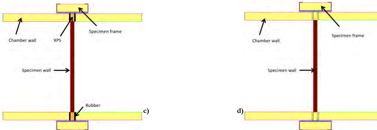
Figure 4.24 – Numerical models of the specimen placed directly: c) surrounded of insulation with 200 mm; d) reference model.
